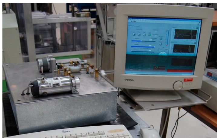
Fig. 1: Motor setup able to reproduce various vibrating environments. The VEPG device under test (blurred) is mounted at the tip of a moving cam.
